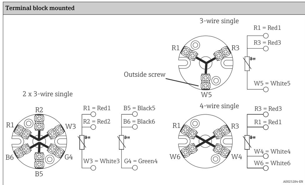
**i** The blocks and transmitters are shown as they sit inside the heads in reference to the conduit opening.
