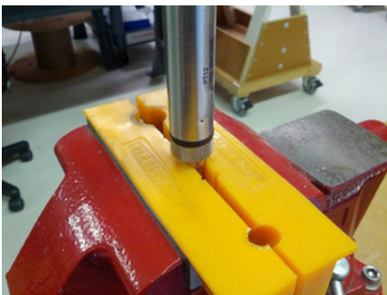
Cabled Sensor - gripping on swage
