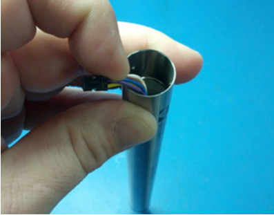
Pull wires gently to the side to allow battery removal.
