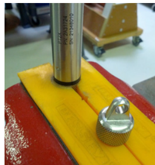
Cableless Sensor - gripping on knurled area
