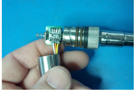
Connector connected properly
