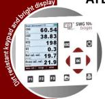
Measuring CH<sub>4</sub>, CO<sub>2</sub>, O<sub>2</sub>, H<sub>2</sub>S (high & low ranges), H<sub>2</sub> and calculated caloric values
