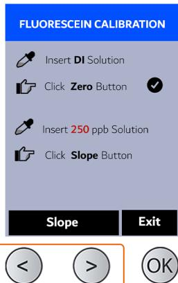
Rinse (3x) and Insert 50 ppb Solution, then select 'Slope'
