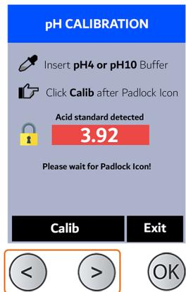
Rinse (3x) and Insert pH10 buffer, wait for lock icon then select 'Calib'
