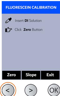
Rinse (3x) and Insert, 250 ppb Solution, then select 'Slope'
