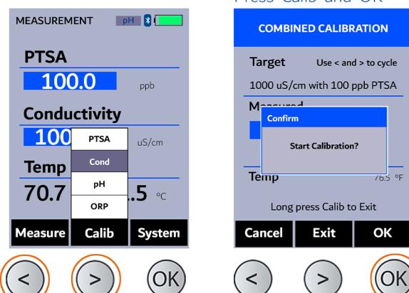
Rinse (3x) and Insert Combined Cal Solution. Press 'Calib' and 'OK'
