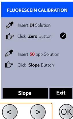
Rinse (3x) and Insert, 500 ppb Solution, then select 'Slope' & 'Exit'
