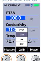
Press 'Calib' and 'OK' COMBINED CALIBRATION Use < and > to cycle 1000 uS/cm with 100 ppb PTSA
