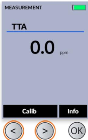
Rinse (3x) and insert TTA Calibration solution. Then press the 'Right Arrow' button to select 'Slope'.
