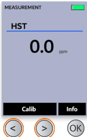
Rinse (3x) and insert HST Calibration solution. Then press the 'Right Arrow' button to select 'Slope'.
