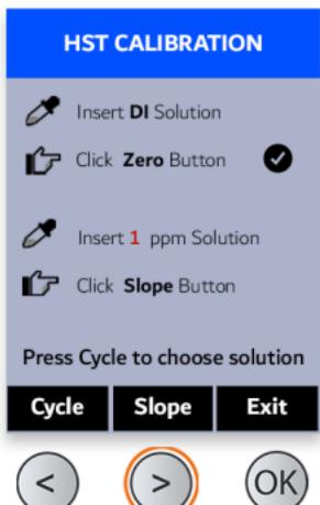
Rinse (3x) and insert DI water. Then press the 'Left Arrow' button to select 'Zero'.
