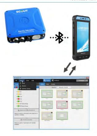
The SCOUT portable connects via Bluetooth to the handheld, which you can then sync with System 1.
