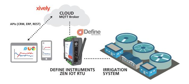
A typical IIoT system uses a broker in the Cloud. I have chosen to use an MQTT broker as it is available in most Cloud systems.
