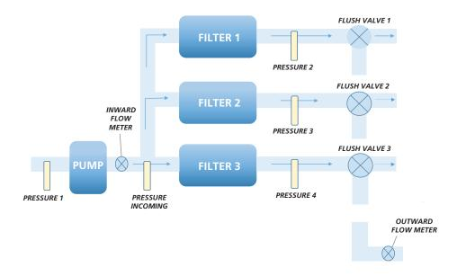
An RTU has been programmed to monitor and control the filtration system and by measuring the differential pressure across the filters, the RTU automatically performs a backflush of the filters when required.
