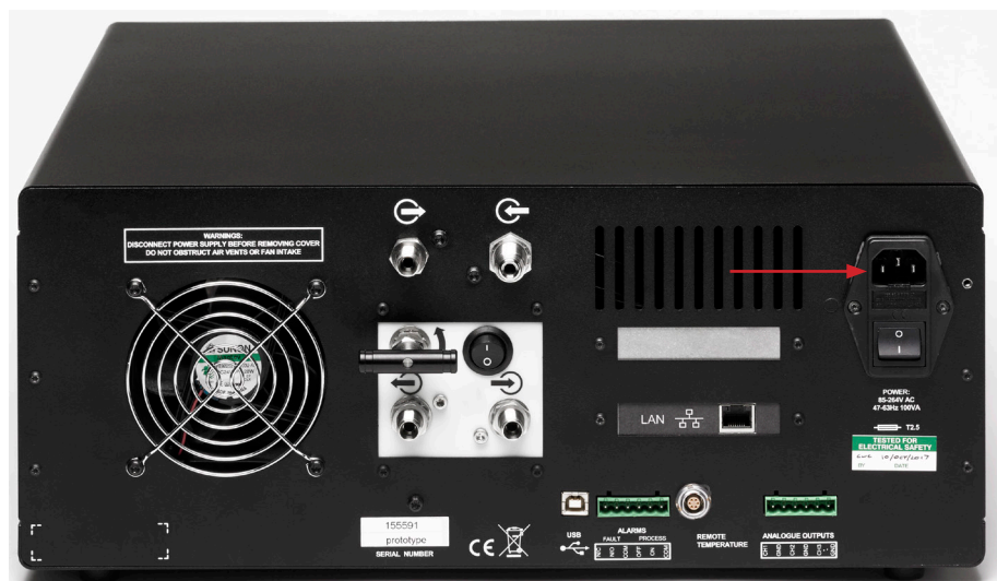
Figure 6 Power Supply Input
