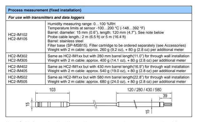
**Note**: HC2-IM1 (120 mm barrel length) - to avoid measurement errors due to temperature gradients fully immerse the probe barrel in the environment to be measured
