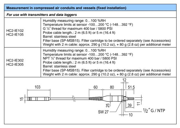
Note: To avoid measurement errors, temperature should be the same on both sides of the mounting wall
