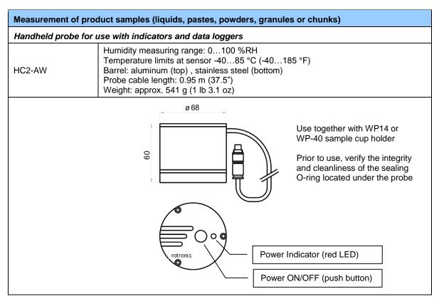
**Note:** When using the HC2-AW probe, check that the red LED on top of the probe is lit. This indicates that the probe is being powered. If necessary, power the probe by pressing once on the red button located on top of the probe. When the red LED is not lit, the probe is not powered and the instrument is not receiving a signal from the probe.
