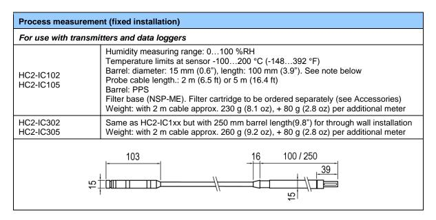
**Note**: HC2-IC1 (100 mm barrel length) – to avoid measurement errors due to temperature gradients fully immerse the probe barrel in the environment to be measured
