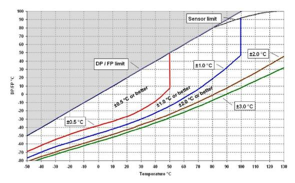
**Example:** at a temperature of 20  $^{\circ}$ C, a dew point value of -37  $^{\circ}$ C is measured with an accuracy of  $\pm$  1.0  $^{\circ}$ C or better.
