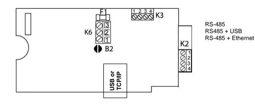
Terminals Description **Terminals** Description K6-1: -► Protective ground K2-4: GND Ground (tied with other GND) Power supply phase: 85 to 240 K6-2 K2-3: GND Ground (tied with other GND) VAC Power supply neutral 85 to 240 K1-3 K2-2: OUT2 Temperature output (+) VAC K2-1: OUT1 Relative humidity or dew point (+)
