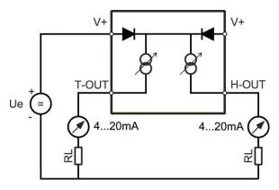
The maximum permissible cable length connecting the HF52 to other devices is determined by the total resistance resulting from the addition of the cable resistance and that of the devices connected in series with the unit. This resistance should not exceed 500 ohms.
