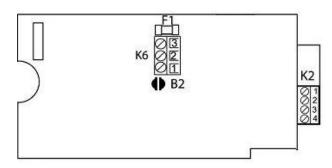
F1: fuse (soldered to PCB)
