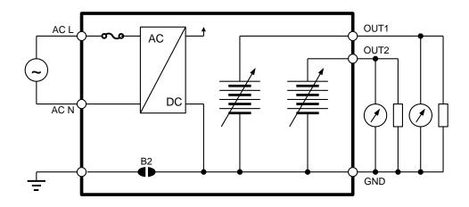
The maximum permissible cable length can be determined under consideration of the voltage drop caused by the current flowing to the devices connected to the unit. The voltage drop in the cable depends both on cable resistance and on the equivalent resistance of the devices connected in parallel to the unit. The total resistance connected to each unit output should be at least 1000 ohms. Cable resistance should not be more than 1/1000 of the load resistance.
