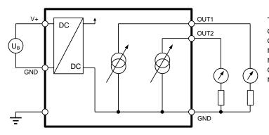
The maximum permissible cable length, connecting the unit to other devices, is determined by the total resistance resulting from the addition of the cable resistance and that of the devices connected in series with the unit. This resistance should not exceed 500 ohms.
