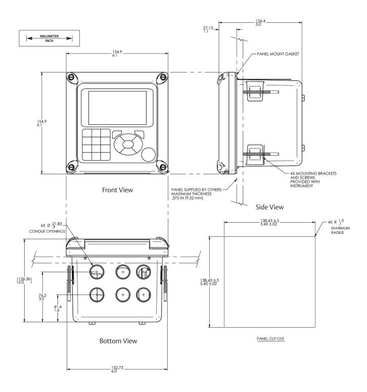
Panel mount dimensions. The front panel is hinged at the bottom. The panel swings down for easy access to the wiring locations.
