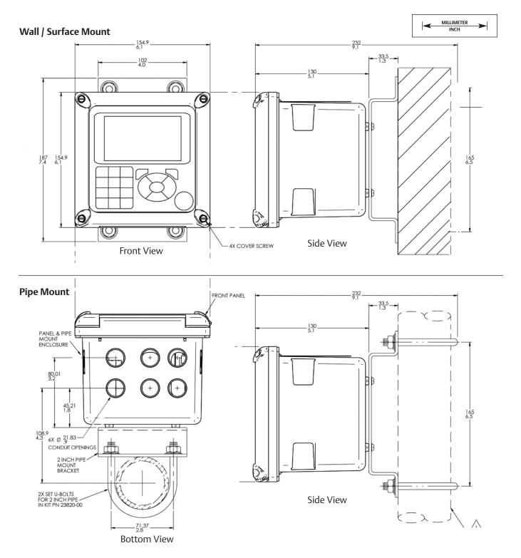
*Pipe/Wall Mount dimensions (Mounting bracket PN:23820-00). The front panel is hinged at the bottom. The front panel is hinged at the bottom. The panel swings down for easy access to the wiring locations.*
