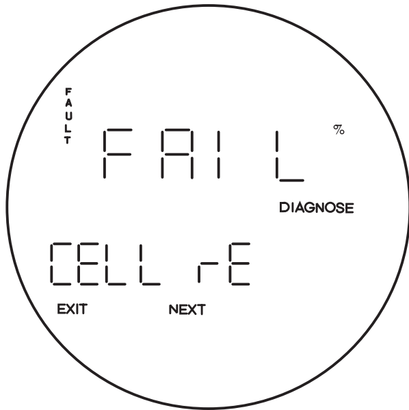
Figure 5-11. Fault 7, Reversed O 2 Cell
