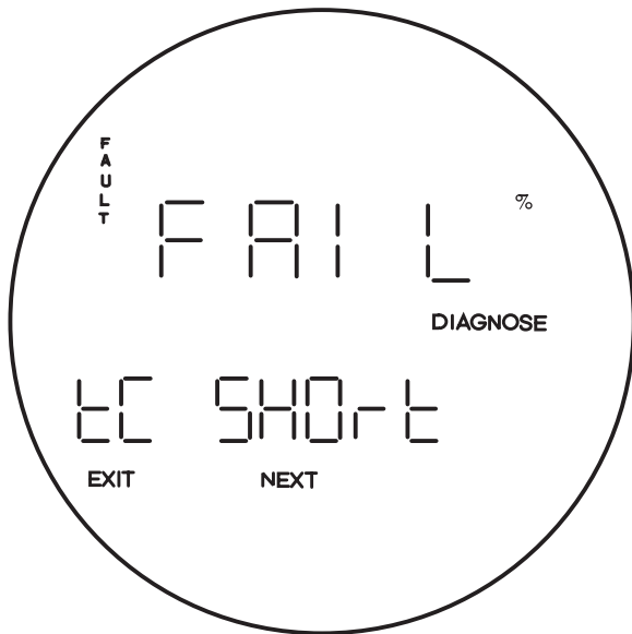
Figure 5-7. Fault 3, Shorted Thermocouple
