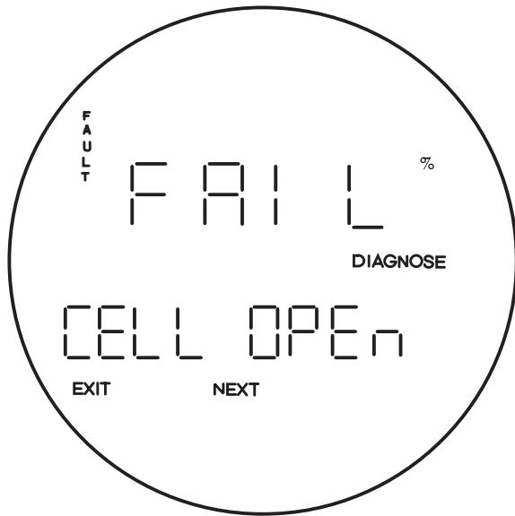
Figure 5-9. Fault 5, O2 Cell Open
