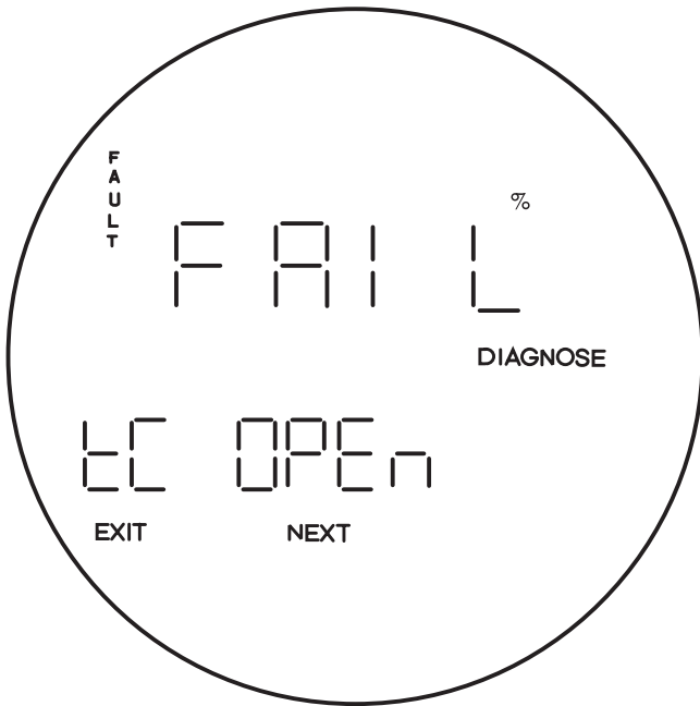
Figure 5-5. Fault 1, Open Thermocouple
