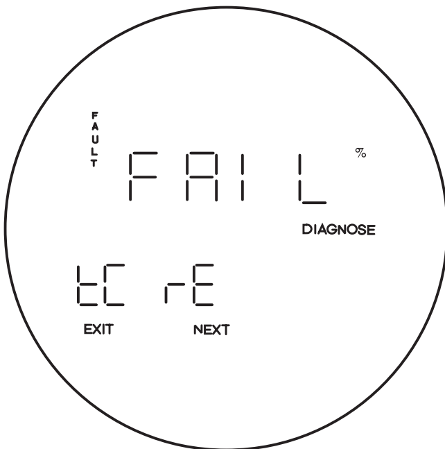
Figure 5-6. Fault 2, Reversed Thermocouple
