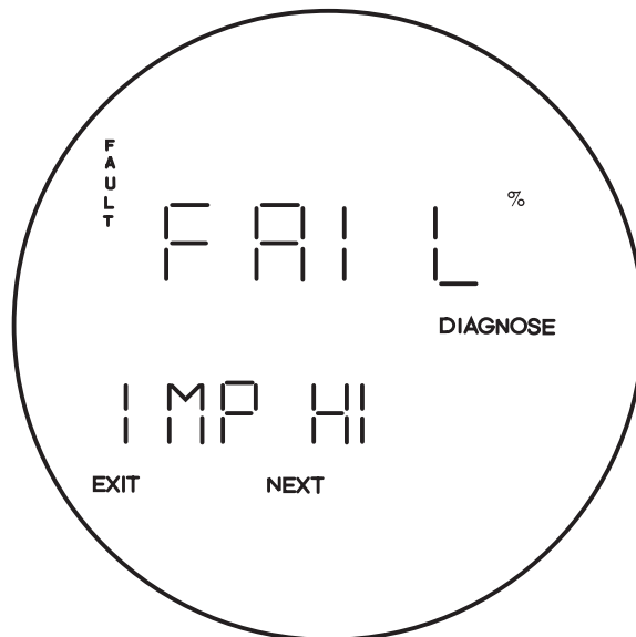
Figure 5-10. Fault 6, Cell Impedance Too High
