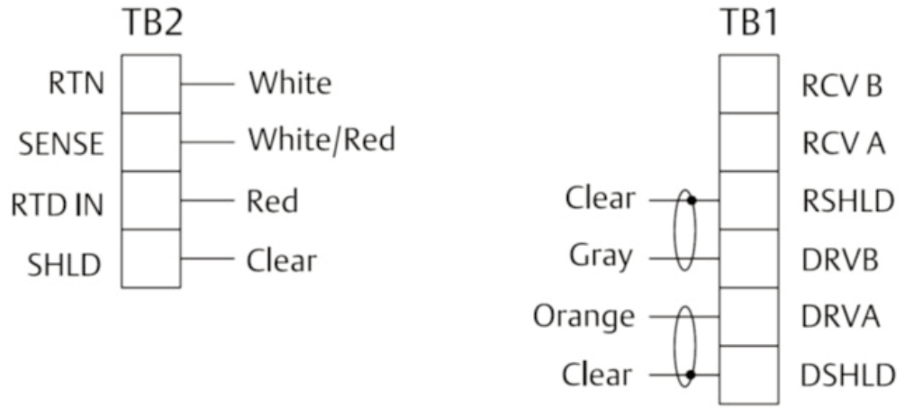
Figure 3-3: Rosemount 403/403VP Sensor Wiring to Rosemount 1066 Transmitter
