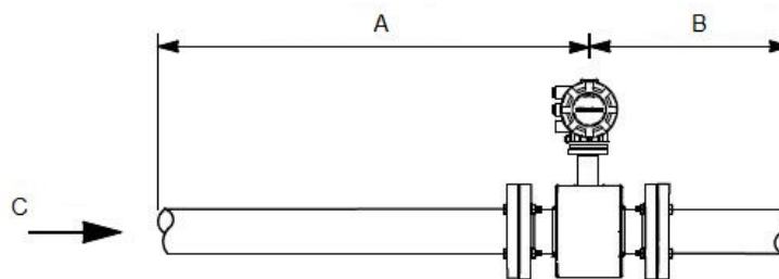
Figure 3-1: Upstream and downstream straight pipe diameters
