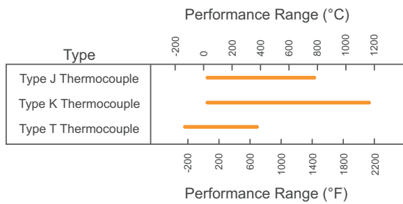
Figure 4: Thermocouple Temperature Ranges
