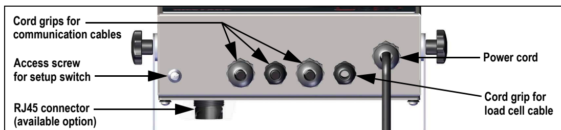
Figure 2-5. Recommended Cord Grip Assignments
