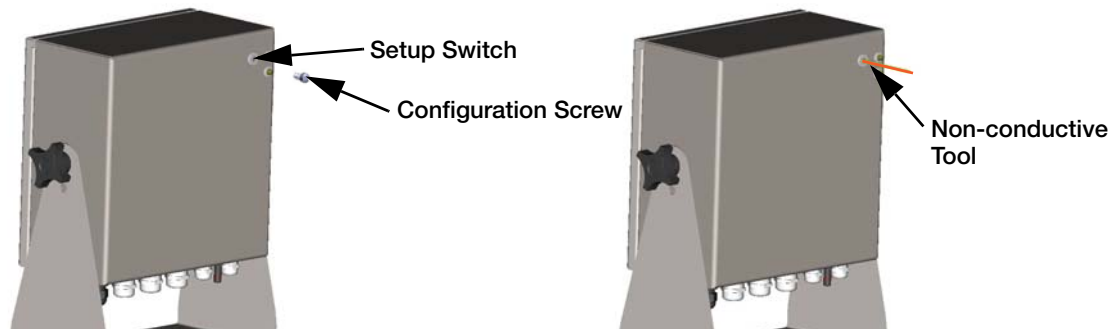
Figure 3-1. Setup Switch Location (Universal Enclosure)
