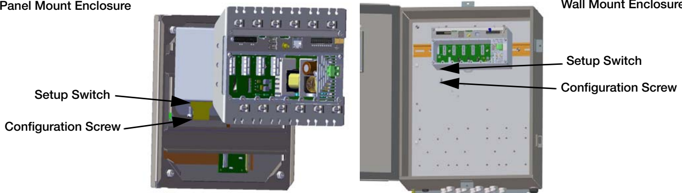
Figure 3-2. Setup Switch Locations (Panel/Wall Mount Enclosures)
