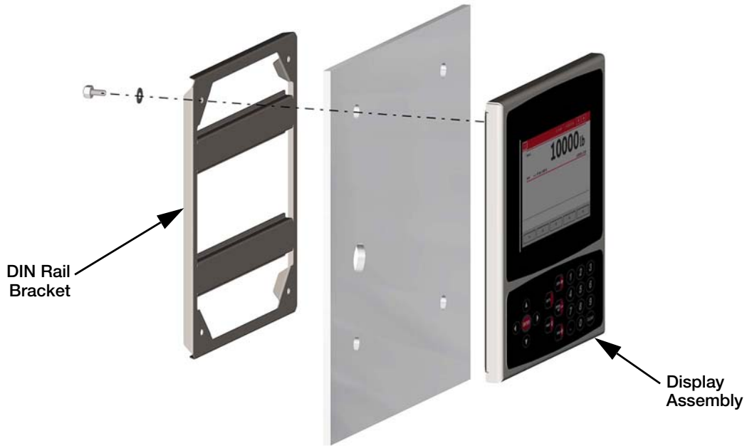
Figure 2-16. Mounting the 1280 – Panel Enclosure
