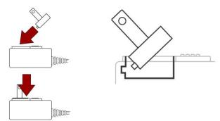
3. Tilt the plug into the adapter's receptacle, aligning the small ledge with the cutout inside the receptacle.
