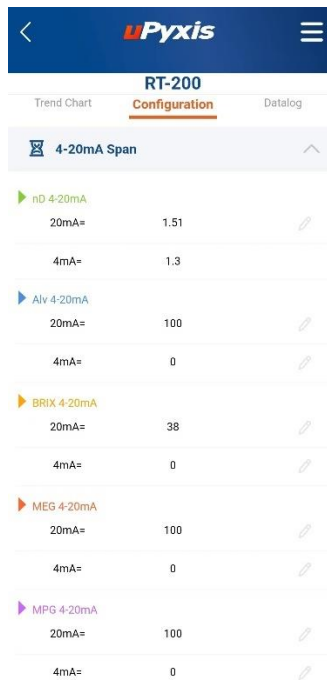
Figure 28. – Setting 4-20mA Range
