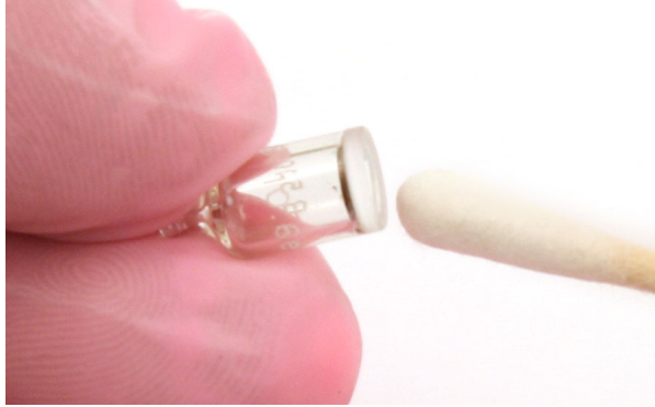
Figure 26: Polishing the Electrode Lamp Window
