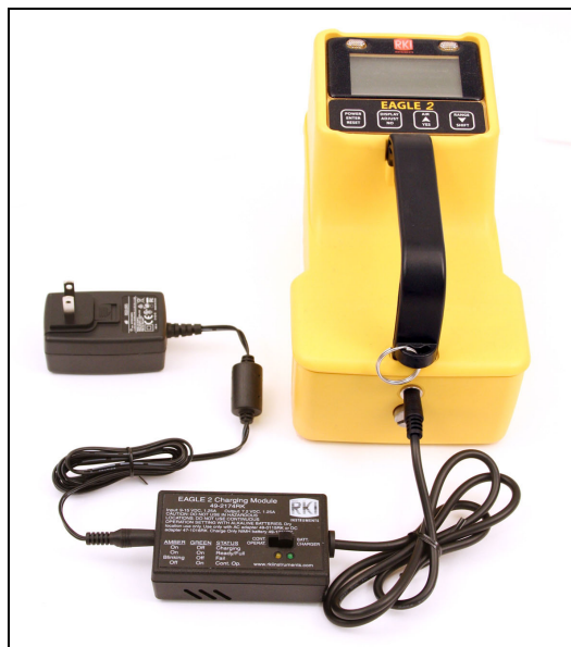
Figure 17: Connecting a Charger to the EAGLE 2
