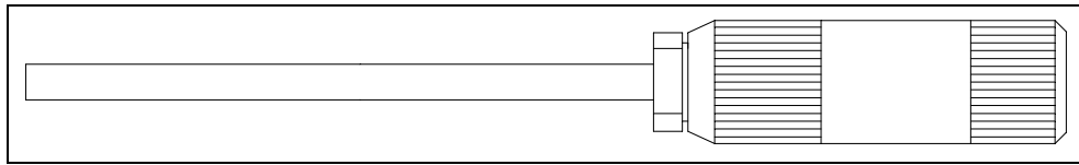
Figure 13: 10 Inch Probe with Dust Filter
