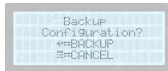
Figure 61: Parameter change triggered backup
