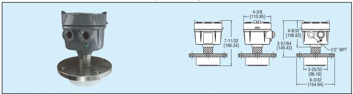
The Model FCLS Flush Capacitance Level Switch is ideal for level measurement of liquids and bulk solids to trigger an alarm or close a filler inlet. No probe design allows for installation where space is constrained or where material flow or material build up would damage a probe. With no moving parts, this level switch assures no jams, no wear, nothing to break, and no maintenance. Comes standard with IP65 housing with a maximum pressure limit of 285 psi (19.7 bar).
