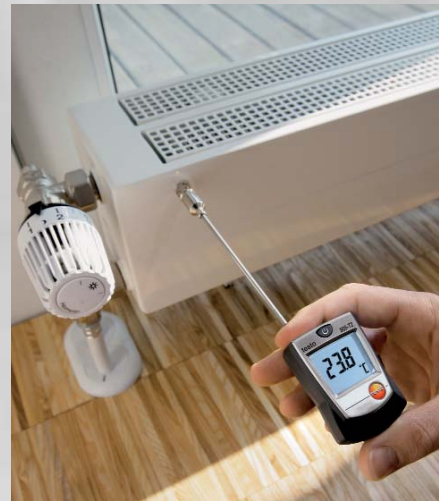
Surface temperature measurement on a radiator
