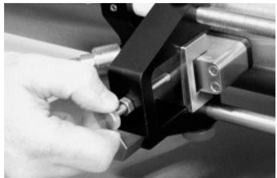
Figure 27: Installing the first transducer
