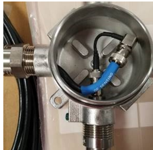
Figure 18: Transducer cable connection with cable jumper, PN133M7313-03
