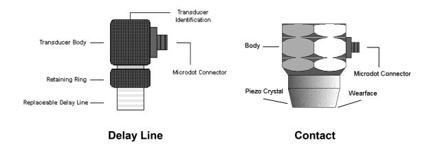
The Transducer is the "business end" of the *PZX-7 DL*. It transmits and receives ultrasonic sound waves that the *PZX-7 DL* uses to calculate the thickness of the material being measured. The transducer connects to the *PZX-7 DL* using a single shielded coaxial cable with microdot connectors.
