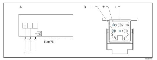
A Electrical connection for devices with Harting plug Han7D
