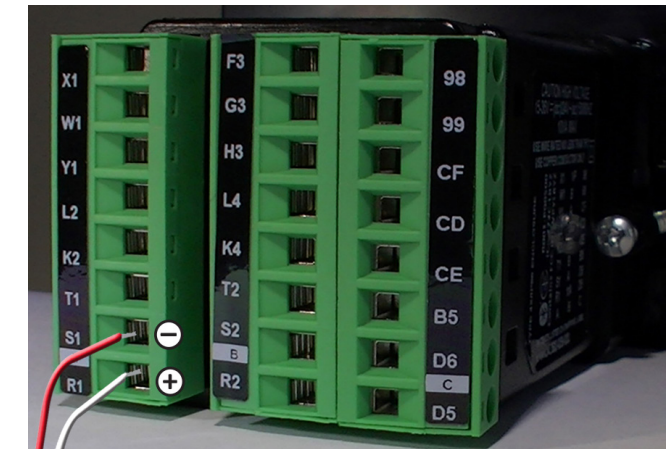
Figure 4: Thermocouple Wiring Example
