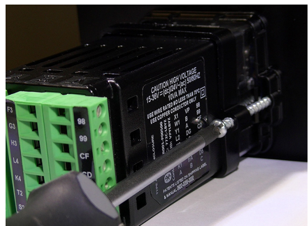
Figure 3: Tighten the Mounting Screws
