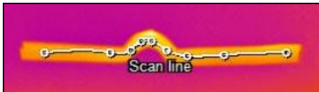
Scan line with multiple points as spline
