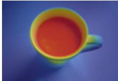
Cross-fading of thermal image and visual image by 50 % setting
