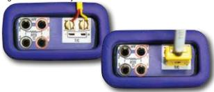
Simulating or reading RTDs uses copper wire.
