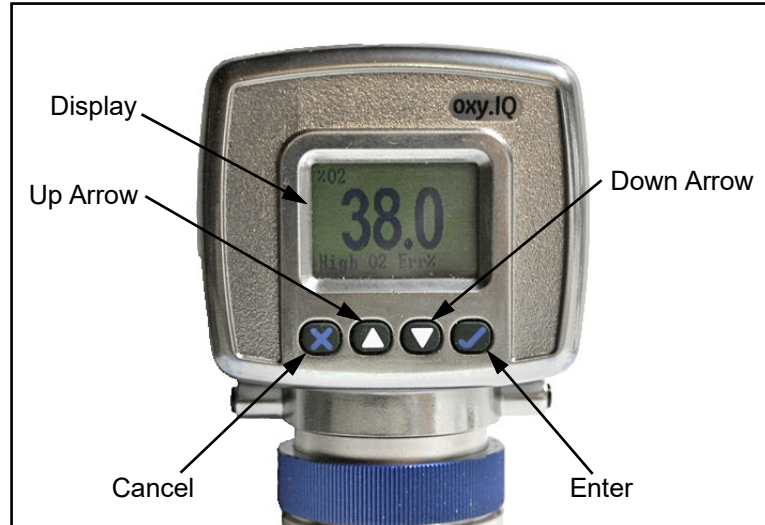
Figure 7: oxy.IQ Display and Keypad
