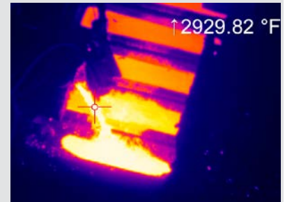
Measurement of a pouring stream.
