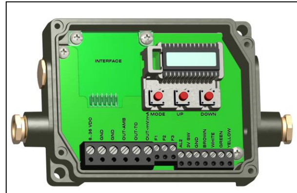
Opened LT/ G5/ P3/ P7 electronic box with terminal connections
