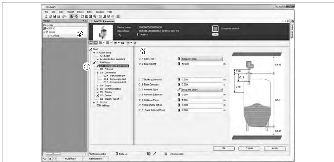
Figure 5-5: Screen from the PACTware™ user interface
