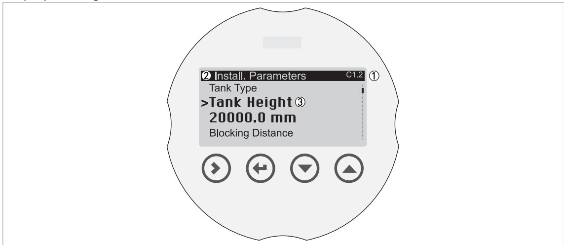
Figure 5-2: Display screen layout in Program mode
