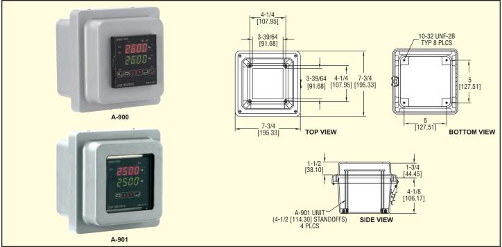
**Models A-900 and A-901** are the perfect instrument housing for indoor or outdoor applications. Protects controls from dirt, dust, oil and water. Unit is rated weatherproof type NEMA 4X (IP66) and has a fully gasketed cover. Standard features include a lockable latch to prevent tampering and flush mounting hardware.
