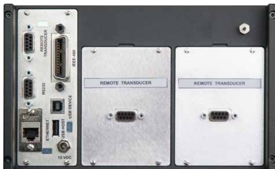
Figure 5.4 B - Two remote transducer interface connections installed
