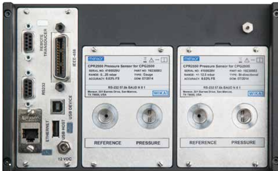
Figure 5.4 A - Two removable gauge transducers installed
