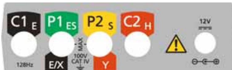
Test lead connections (at rear of instrument)
