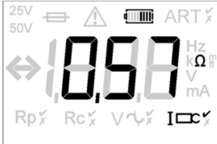
Figure 36: example resistance reading using two-clamp stakeless method
