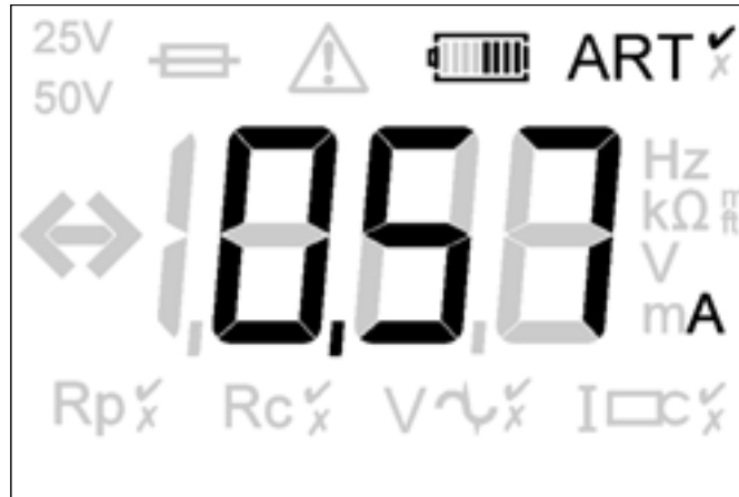
Figure 30: example ground current reading (DET4 display shown)
