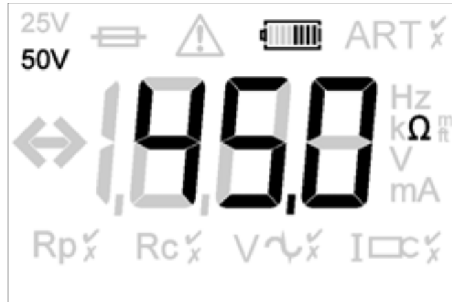
Figure 14: example two-terminal resistance reading (DET4 display shown)
