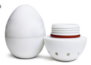
The EGMS comes with a humidity and temperature cap, and a temperature only cap. The temperature and humidity cap is vented to measure humidity, where as the temperature only cap is not vented making the product submersible.
