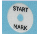
To start the device, hold the magnetic wand over the start/mark switch.
