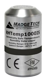
the RHTemp1000IS, allows it to be placed in remote or hard to reach locations. The device now features a battery life indicator allowing users to easily identify low voltage and change batteries when required. This feature maximizes the use of your battery life and is a cost saving efficiency. The RHTemp1000IS can hold up 16,350 humidity and temperature measurements. Its real time clock ensures that all the data is time and date stamped.
