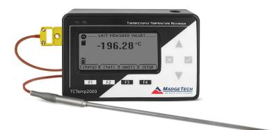
MadgeTech's LNDS, Liquid Nitrogen Data Logging System, is an ultra-low temperature measurement system created specifically for the monitoring of temperature sensitive substances that need to be preserved at cryogenic temperatures.
