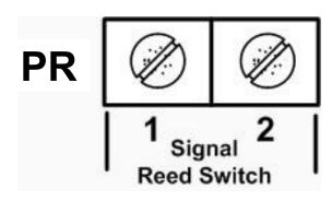
The PR unit cam only accept a reed switch input, this sensor has been selected as the most common sensor and requires very little power with small effect on battery life.
