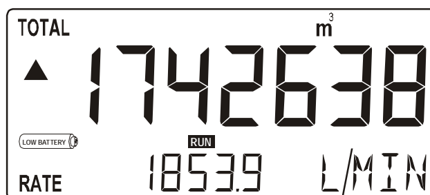
Fig. 4: Example of low-battery alarm.
