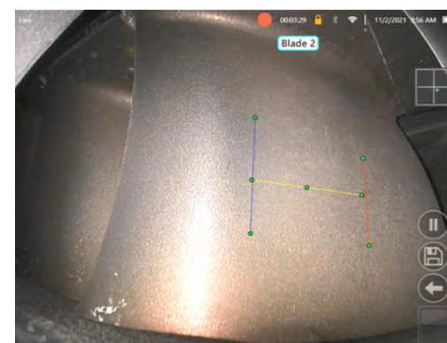
Fig 9c. Blade Counter active showing original tracking region
