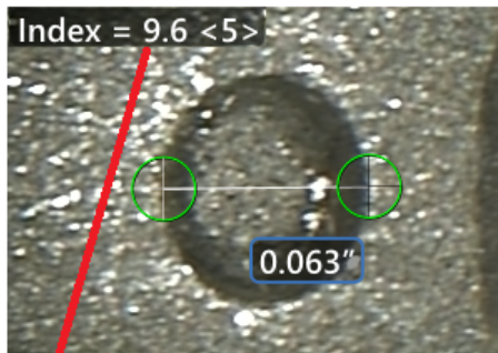
The stereo index can be displayed to indicate the amount of magnification you have achieved.
