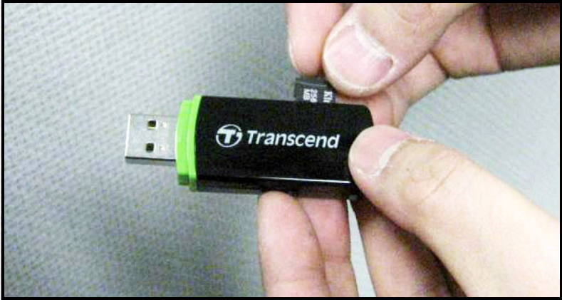
Figure 55: Plugging the Reader into a PC
