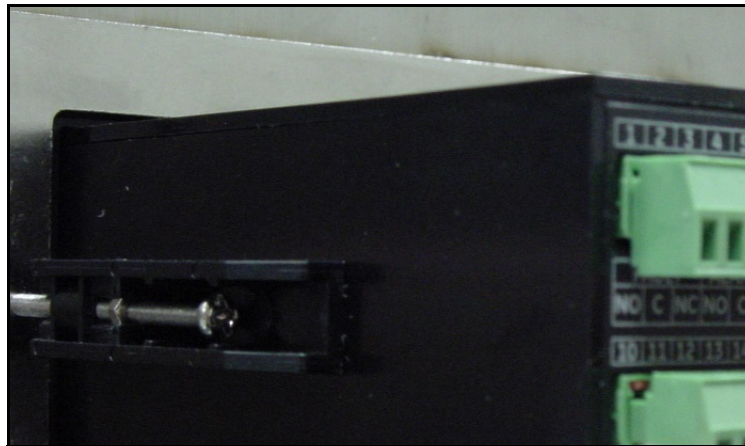
Figure 36: Reinserting the Connector into the Terminal Block
