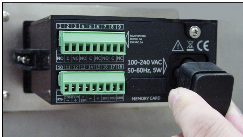
Figure 38: Inserting the AC Power Cable
