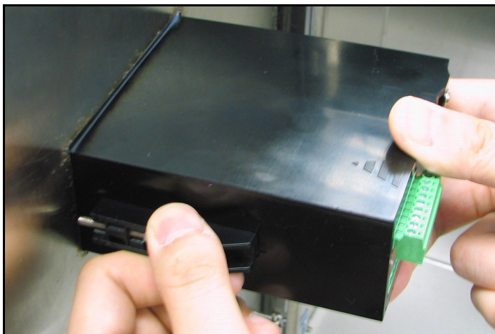
Figure 13: Locking the Mounting Brackets in Place
