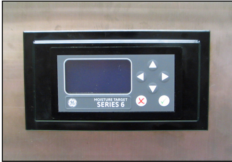
Figure 22: MTS6 Installation with Adapter Plate – Front
