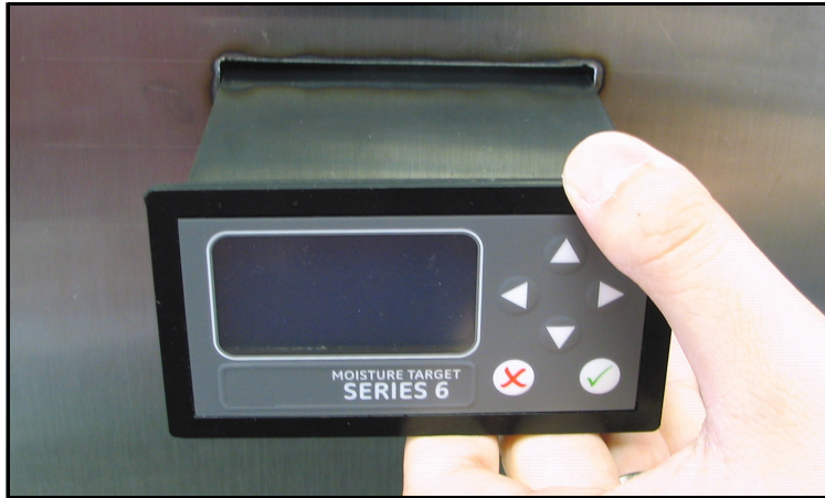
Figure 11: Sliding the MTS6 into the Panel Cutout
