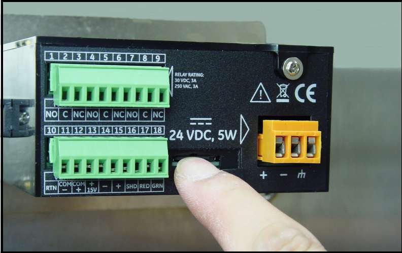
Figure 53: Pushing in on the MicroSD Card
