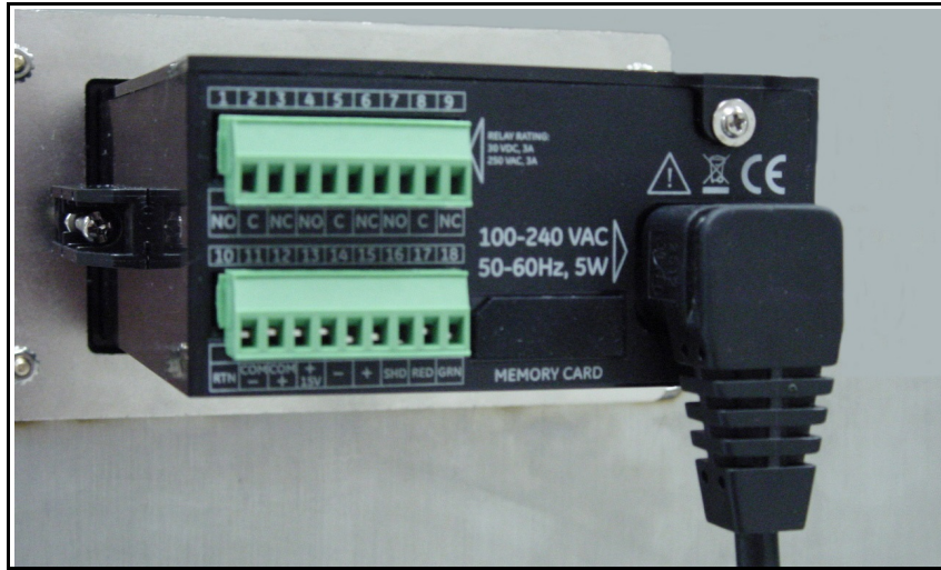
Figure 39: The AC Power Cable Installed
