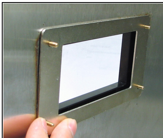
Figure 18: Applying the Backing Plate
