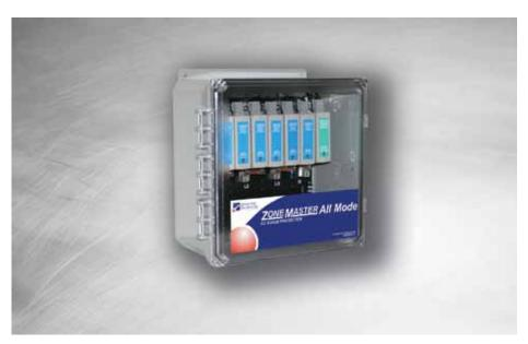
Large block Metal Oxide Varistor (MOV) protection technology is utilized within the ZoneMaster All-Mode range. Each of the large block MOVs are individually fused for both thermal and short circuit protection. This produces redundancy ensuring the facility is never unprotected.
