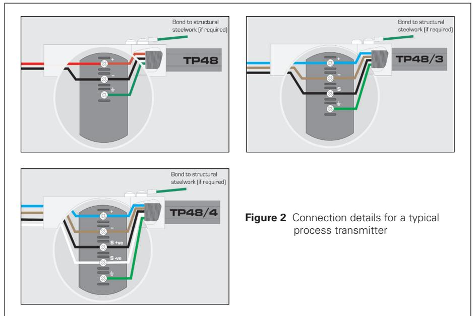
Figure 2 Connection details for a typical process transmitter
